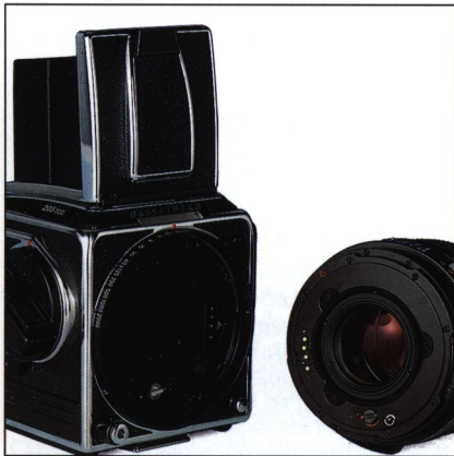
The four electronic contacts between lens and camera body.
