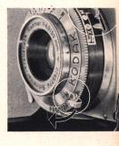
Since the "X" setting provides synchronization for Class F flash lamps, the self-timer can be used for flash pictures with SM or SF lamps.
