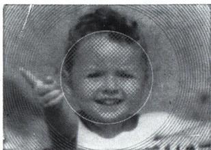
Microprism screen is fuzzy = unsharp
