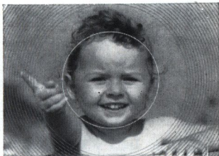
Microprism screen not fuzzy = sharp
