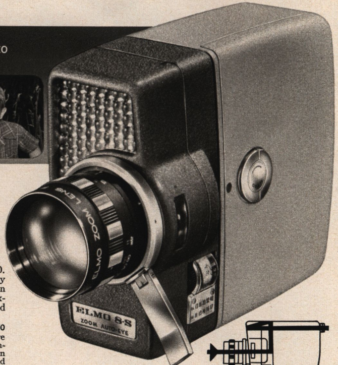
Focus and view with through-the-lens finder. Single-lens half-mirror reflex system eliminates parallax
