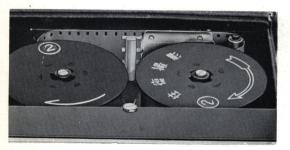
Turn over the loaded spool so that the Figure 2 is visible, and then insert it in the upper spool stud. Then, repeat the procedure given on Page 4.
