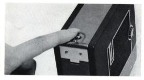
Push the Battery Compartment Cover Button and the Cover will swing open.
