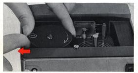
Hold footage counter lever down and remove take-up spool.
