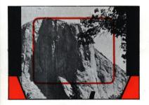
Yashica 8-ES with an universal focus lens does away with the trouble of focusing and is set at the standard speed of 16 frames per second. The red frame in the finder outlines the exact area which will appear on the film. Always make sure to compose your picture within this frame.
