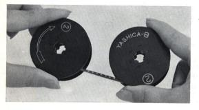
Using the Second Half of the Film. After filming the full 25 feet, run the film until the red indicator of the footage counter aligns with the "E" mark. Then, open the side cover and remove the spool from the take-up spool stud, taking due precautions against recoiling of the film.
