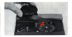
Pull out about 6 inches of film leader. Set spool on upper spool stud and slip film in front of spring-loaded pressure plate. Make sure the film is threaded according to diagram in the camera and rests on the guide rollers beside the pressure plate.
