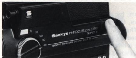
To adjust the viewfinder to your eyesight, turn the diopter control dial, while looking through the viewfinder, to a position where you can see the aperture indicator as clear as possible, then set it at that position.
