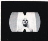
B. Press the Hi-Focus button so you can see the double image through the viewfinder as shown in the illustration.
