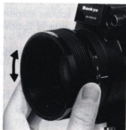
8. The lens ..... correctly focused. Check by pressing the Hi-Focus button.
