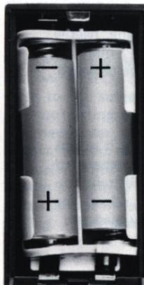
After folding out the pistol grip, open the battery compartment and take out the battery case. Insert four pen-light Mallory MN-1500 or Eveready E91 Alkaline batteries as indicated inside the case. Be sure that the polarity position of the batteries is correct according to the positive (+) and negative (-) diagram inside the case.
