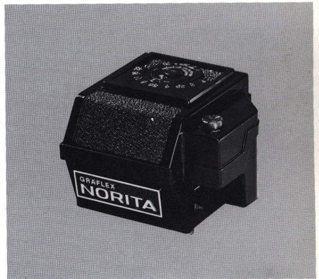
Cat. No. 7963 Pentaprism with Meter is coupled with the shutter speed selection knob as an averaging metering system. The measured range weighted 60% for the area covered by the circle in the center of the focusing screen circle. ASA Film Index—32 to 6400. Uses PX77 or S-76. Battery is supplied.
