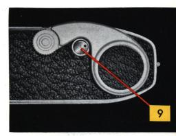
To rewind the exposed film depress the reversing button (9) in the base of the camera, and half pull out the rewind knob (7) to its first stop (see page 16), to get at it more easily. Then turn the rewind knob in the direction of the arrow until the reversing button (9) ceases to rotate. This button carries a black dot near its edge for easier observation.
