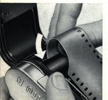
The narrow slit of the take-up spool must point upwards to take the beginning of the film. If necessary turn the take-up spool with the finger or by a few short movements of the rapid winder into the correct position. Then:
