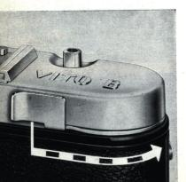
One full movement of the rapid winding lever, as far as it will go, tensions the shutter, and advances the film and film counter. The spring returns the lever to its original position each time.
