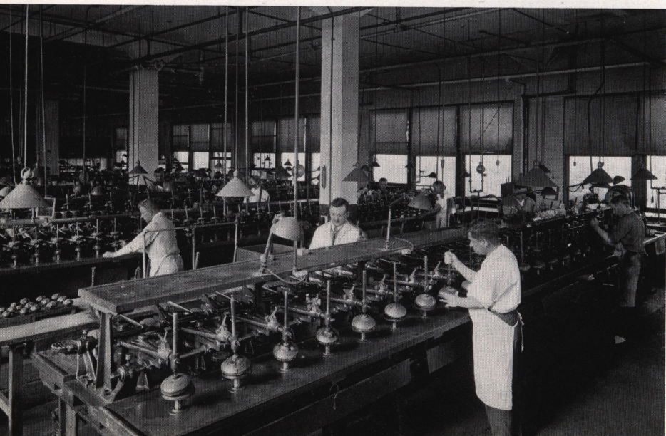
Machines which grind and polish lenses.
