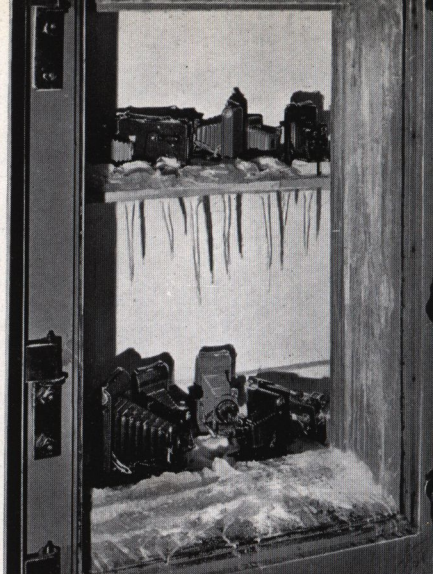
The cold tester. Materials and occasional finished cameras "off the line" are subjected to conditions saltier than Atlantic City, colder than Spitzbergen, and damper than London.
