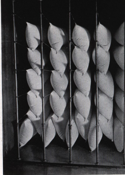
Filter bags eliminate dust from the air that will dry sensitized film. . . . Despite the external cleanliness of Kodak Park, frequent changing of these lintless cotton flannel bags is necessary to maintain the standard for air supply.
