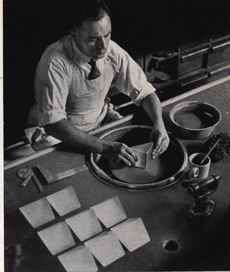
Grinding special prisms, a work that requires a high degree of skill.
