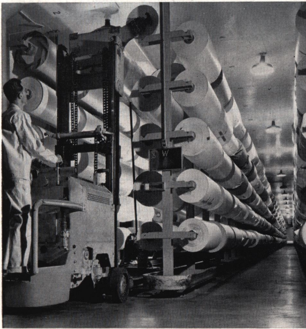
Baryta-coated paper awaiting sensitizing. Handling of the 275-pound rolls is accomplished by specially designed electric trucks.
