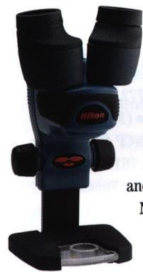
Designed to view extremely small subjects in their natural state at close range. Nikon's new 20x stereoscopic Naturescope can also be used in numerous close-up viewing applications in the home, office or laboratory. Features include an 11mm field of view, 12.6° angle of view, pivoting ocular eyepiece, diopter adjustment, internal 2.5 lumen halogen light and tripod mountable base.
