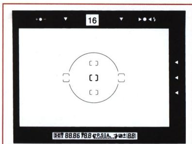
**NIKON'S F5 OFFERS AUTOFOCUS WITH A UNIQUE CROSS-TYPE ARRAY OF FIVE FOCUS DETECTION SENSORS.**
