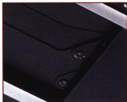
With the Nikon F4s, this multi-blade curtain has been doubled, leaving virtually no room for light leaks. You can perform mirror lockup shooting without the fear of light leakage.
