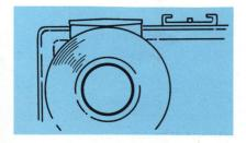
When positioned correctly, the smaller opening of the Eye Shield fits snugly over the raised boss of the focusing window, preventing Shield movement.
