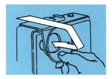
Pull backward on the body of the Eye Shield and fit the remaining lip over the rear edge of the rangefinder housing. The opening of the Eye Shield should now be positioned over the circular focusing window.
