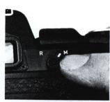
You've got to cock multi-exposure lever for each additional exposure on frame—it returns to central position when you press shutter release.
