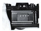
Interior's nicely finished and Rollei's own 14-blade metal shutter's accurate, fairly quiet.
