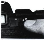
You've got to cock multi-exposure lever for each additional exposure on frame—it returns to central position when you press shutter release.
