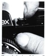
Move electronic self-timer off "0" and red light at thumb stays lit while timer's timing.
