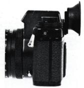
You've gotta slide eyecup up before you can swing back open to load camera.
