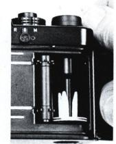
Small "sprocketed collar" atop "regular" sprocket shaft is self-aligning, controls exposure counter (see text).
