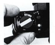
Two-stage ASA setting's less convenient. First you set ASA in window, then release and turn outer dial to align number with white index mark.
