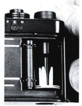
Small "sprocketed collar" atop "regular" sprocket shaft is self-aligning, controls exposure counter (see text).
