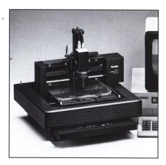
reseau crosses can be transformed onto the calibrated reseau field of the camera. These picture coordinates are stored on the MR2 files and can then be further processed using the MR2-System.
