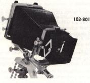
KARDAN-COLOR 8x10" camera with two-section 26" monorail. Front and back standards with geared, self-arresting vertical adjustments; 8x10"/ 26" bellows; 8x10" Universal Back. Supplied with hinged tripod base and flat adapter frame for lenses mounted on Linhof 5x7 (5.1/16" square) lensboards.
