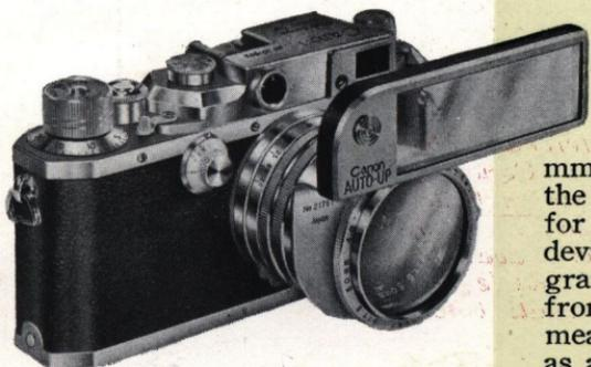
Similar to IV-S(2) but with speeds from 1 sec. to 1/500 sec., B, T and X. This model is also available with the Canon 50 mm f:3.5 lens. Also shown is the Canon Auto-up attachment for the 50mm f:1.8 lens. This device permits close-up photography between 22" and 40" from the camera. Actual measurements are unnecessary as all focusing is done through the camera body rangefinder mechanism.
