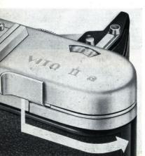
One full movement of the rapid winding lever (see illustration) transports the film and at the same time advances the film counter. The spring action then returns the winding lever to its rest position. The rapid winding lever can of course also be worked in a number of short movements. In that case carry on pulling it until it comes to a distinct stop.
