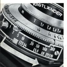
The iris diaphragm of the lens controls the amount of light reaching the film — and thus inderectly the exposure as well as the extent of the depth of field. Set the aperture by moving the aperture lever (7), so that the lever lies against the line corresponding to the required aperture number (see illustration).
