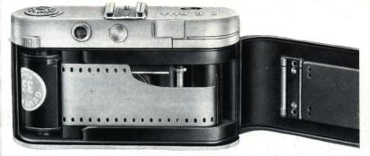
The illustration shows the correctly loaded camera before closing and setting the film counter. The rewind knob is pushed down into the body, and the film lies flat in the film track. Then fold down the camera back and press it against the body; make sure that the locking ledge engages properly.
