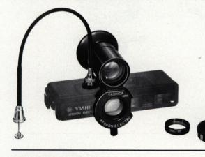
Set consists of two lenses, exclusive viewfinder, cable release and scale. Selective use of the two lenses enables close-ups at ranges of 20cm (8 in.) and 40cm (1 ft 4 in.). An indispensable aid in copying documents, etc. Provides effective coverage of an area of 9.7 x 7.1cm (3.8 x 2.8 in.) from a range of 20cm; 21.5 x 15.6cm (8.5 x 6.1 in.) from a range of 40cm.
