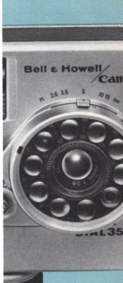
Since the SE 28mm f/2.8 lens has a relatively deep depth of field, you can be quite sure of getting sharp pictures by employing the Zone, Focus System (Method B).
