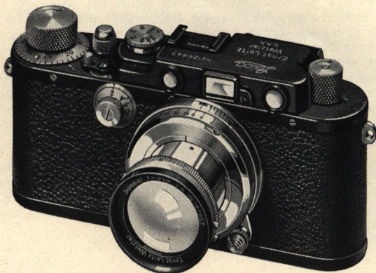
Fig. 1 LEICA Model F with built-in range finder, coupling for automatic lens focusing, and shutter speeds between 1 second and 1/500 second. SUMMAR f:2.5mm lens on camera
