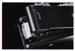
**REWIND STOP**Film rewind automatically stops when finished.
