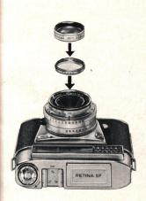
Screw the R close-up lens in front of the basic lens of your RETINA camera. The mark on the R lens must conform with the mark on the gauge rods used. For gauge rods 1.5 combine the R 1:2 and R 1:4.5 lenses and screw the combined lenses to the camera, the R 1:2 lens next to the camera lens. Filters are screwed to the R close-up lens.
