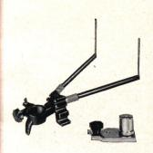
Introduce two gauge rods of equal denomination, say No. 2, into the guide grooves of the attachment identified with the same number and tighten the thumb nuts. The rod marked with a small circle goes on the side of the attachment also marked with a circle. Gauge rods 2 and 1.5 have two guide grooves in common.
