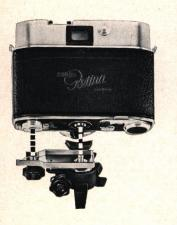
Place your RETINA on the camera holder. Make certain that the guide pin is in the guide hole in the camera bottom. Secure the camera with the tripod screw.
