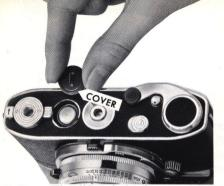
**Battery**—The life of the battery, supplied, is approximately two years.\* To replace the battery, turn the coin-slotted battery COVER counterclockwise, move the milled lever aside, and remove the cover. Remove the used battery and replace it with a PX-13 type *mercury* battery, inserted with its *positive side* (+) *toward the inside*, Replace and fasten the cover by turning it clockwise. \*With average use.
