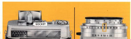
4. Lens Opening-From the Flash Guide Number table, opposite, select the proper flash guide number for the film you are using; divide this number by the camera-to-subject distance in feet (found in step 3) to find the nearest lens-opening number. Rotate the lensopening scale by its black handles until this number is opposite the index mark. For example, if KODACHROME-X Film were loaded in the camera.
