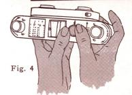
operated with the thumbs. (Fig. 4) STEP 3: Make sure that wind knob (A), its shaft (S) and the film spool (R) are all coupled together. The small "pin" (Fig. 5) fits into the slot in the wind knob shaft (S). Both spool and knob should be locked against rotation. STEP 4: Push the release button (B) in the direction indicated by the arrow above it and revolve the sprocket (P)
