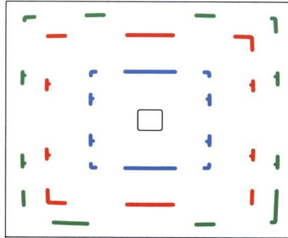
For illustrative purposes only, this diagram shows the frame lines of the various lenses in color: 65mm-green. 80mm-orange. 150mm-blue. The viewfinder shows only one automatically indexed frame line at a time, in white.
