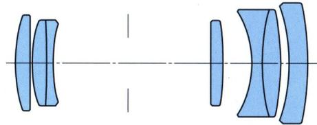
1. Weight of 480g (16.9oz.) and filter diameter of 58mm. 2. Lens elements of low-dispersion glass assure maximum correction of chromatic aberration for exceptional image fidelity. 3. This telephoto lens is a compact companion to the 150mm, designed for aerial or landscape photography and other applications. 4. The extended reach, coupled with its compact, lightweight design, provides particular versatility and superior performance.
