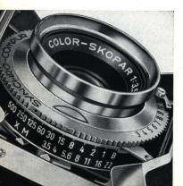
carries shutter speeds of 1, 1/2, 1/4, 1/8, 1/15, 1/30, 1/60, 1/125, 1/250, and 1/500 second as well as "B" for time exposures. It is speed-synchronized for all types of flash, and fitted with a built-in delayed action release (self-timer).
