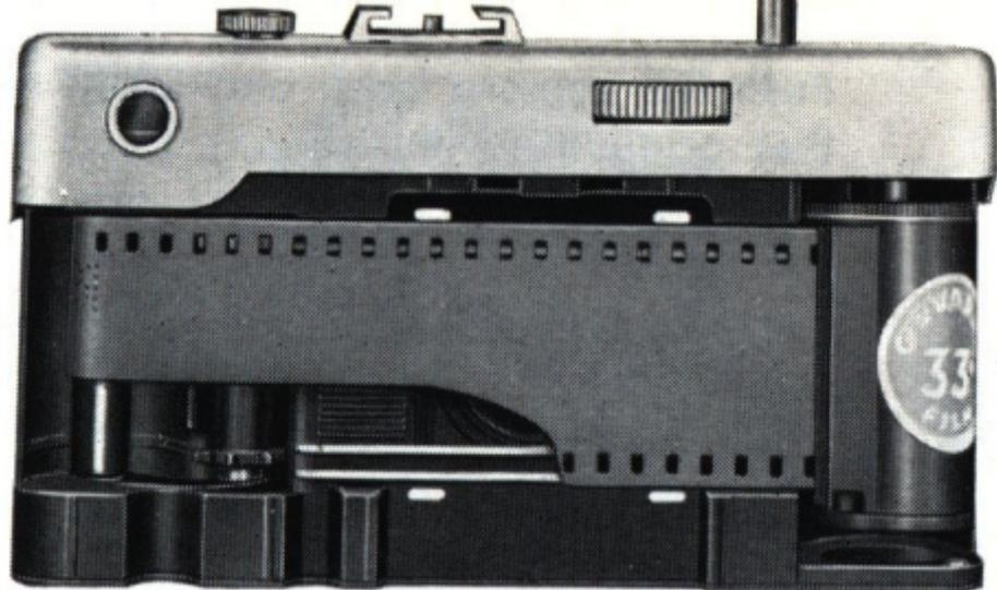
Once the film is in position in the camera as shown in the illustration, first set the film counter mechanism and the film indicator, and close the back. Do this as follows. Hold cartridge in position and turn the camera over. Rotate film counter disc until the diamond  $\blacklozenge$  mark is next to the index line. Set film indicator by rotating.
