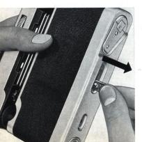
like unloading and changing partly exposed films (see pages 22 and 23) is specially easy and quick, for the camera back is separate from the body. You can therefore remove it completely and carry out all the necessary operations without obstruction.
