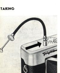
To take the picture, gently but smoothly press the release button. Do not jerk it or stop half-way. Short instantaneous exposures ( $^{1}/_{30}$  second or faster) are usually taken with the camera held in the hand. Avoid holding the camera unsupported for exposures longer than  $^{1}/_{30}$  second; prop up your arms or lean your body against something solid.
