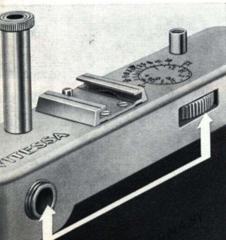
combines a viewfinder and rangefinder in one. On looking through the eyepiece (arrow, left) you will see the finder image with the bright rangefinder field in the middle. On the right, within comfortable reach of the right thumb, you will find the milled focusing wheel.
