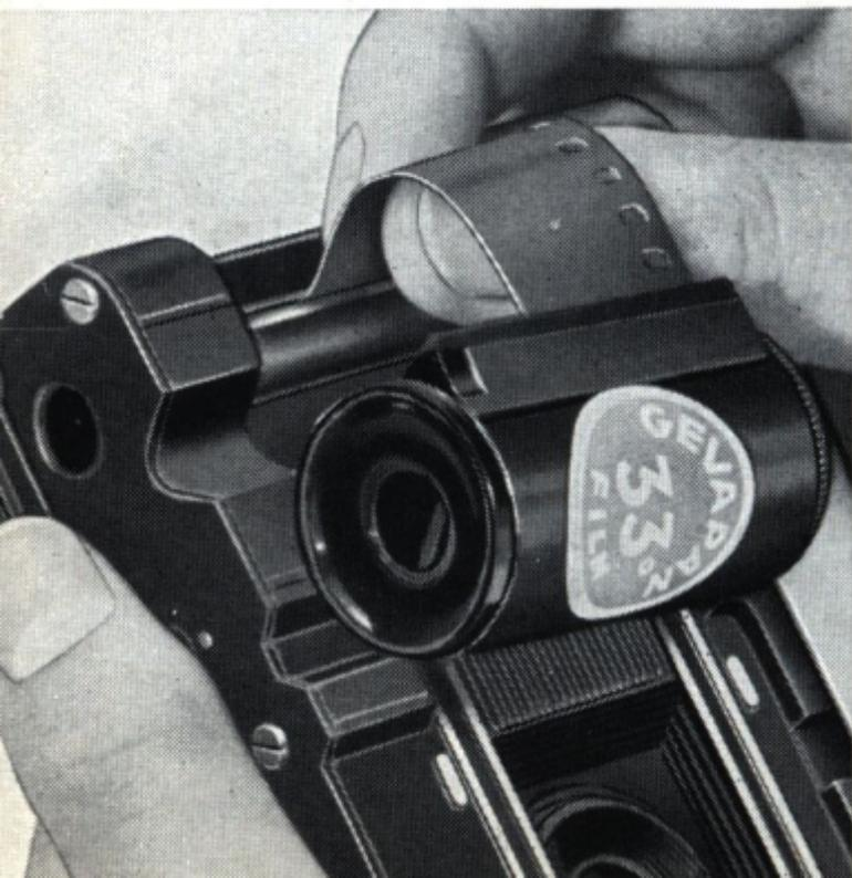
The VITESSA takes standard daylight cartridges of perforated 35 mm. film. Although these cartridges are light-tight, it is best not to handle them in too strong light. Therefore load and unload the camera in the shade — even the shadow of your own body will do.
