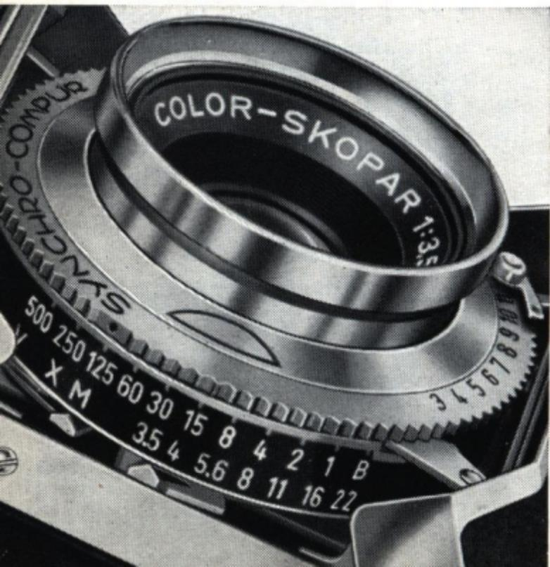
carries shutter speeds of 1,  $\frac{1}{2}$ ,  $\frac{1}{4}$ ,  $\frac{1}{8}$ ,  $\frac{1}{15}$ ,  $\frac{1}{30}$ ,  $\frac{1}{60}$ ,  $\frac{1}{125}$ ,  $\frac{1}{250}$ , and  $\frac{1}{500}$  second as well as "B" for time exposures. It is speed-synchronized for all types of flash, and fitted with a built-in delayed action release (self-timer).
