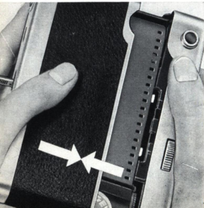
Push the camera back and body together again (see illustration). Keep them pressed together while you turn back the latch and fold it down.
