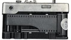
Once the film is in position in the camera as shown in the illustration, first set the film counter mechanism and the film indicator, and close the back. Do this as follows. Hold cartridge in position and turn the camera over. Rotate film counter disc until the diamond  $\blacklozenge$  mark is next to the index line. Set film indicator by rotating.
