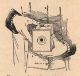
5. Press the Button.—To do this without swaying the camera to one side, grasp the Kodak as shown in the cut, with the left thumb on the button and the ends of the fingers around the corner of the box, giving a leverage whereby the button can be depressed by a muscular contraction of the hand, as in the preceding cut.
