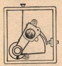
FIG. 3-POSITION OF SHUTTER AFTER INSTANTANEOUS EXPOSURE.
