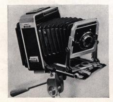
Forward tilting lensboard and drop bed combine for 30° tilt. Increases apparent depth of field when taking pictures from a balcony, down a flight of stairs or in similar situations. Drop bed also accommodates wide angle lenses.
