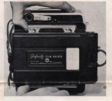
New style double cam action slide lock holds any accessory for Graphic or Graflok back. Slide off focusing panel and attach Grafmatic sheet film magazine, Roll Film Holder, Film Pack Adapter, Polaroid Back or Graflarger. Accessories become part of the revolving back.
