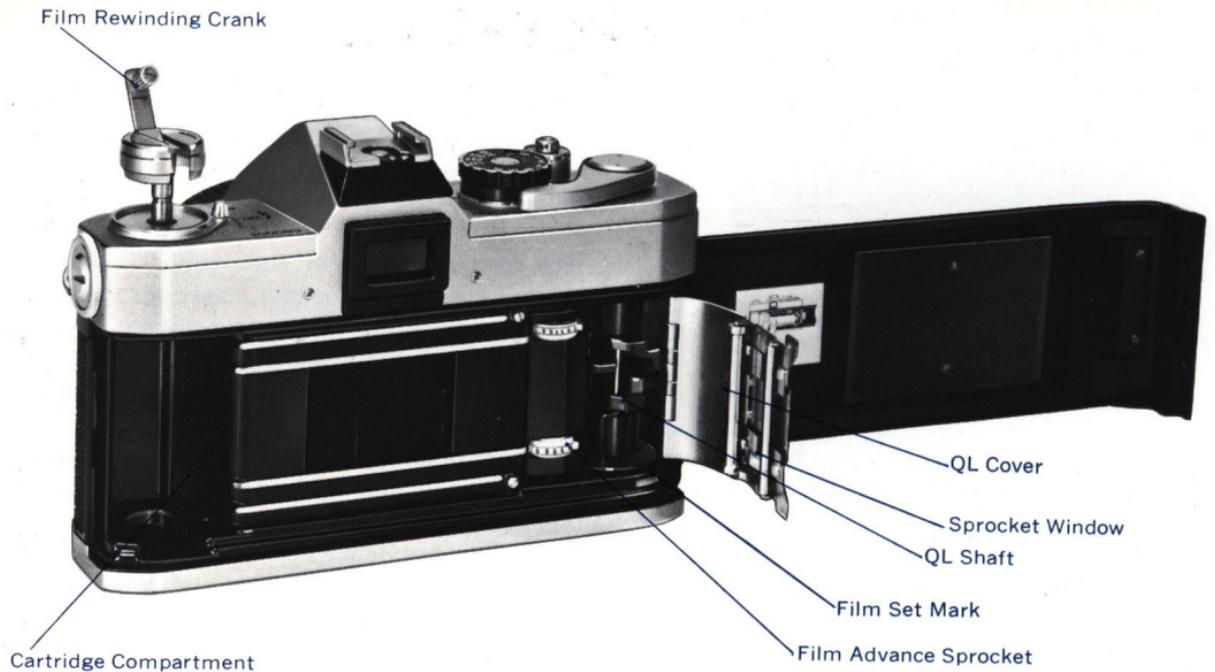
Position in which film is placed in camera
