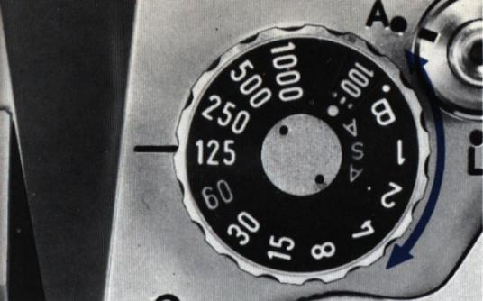
**5** If the meter needle is pointing above the meter index and cannot be matched by closing the preset aperture ring and metering cannot be performed, turn the shutter speed dial to the faster side. If the meter needle is pointing below the meter index and cannot be matched by opening the preset aperture ring, turn the shutter speed dial to the slower side. When the red signal appears, use high-speed film or the Canon Booster.
