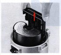
**3.** Remove the C-type battery cartridge <sup>(5)</sup> from the battery chamber.
