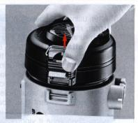
Unlock the silver buckle catches from the pins on the speedlight case and pull up on the battery chamber cap.
