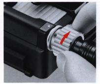
Check the O-ring: Before connecting the camera plug to the camera, examine the plug's O-ring for dust and scratches and be sure it is properly seated and lubricated.
