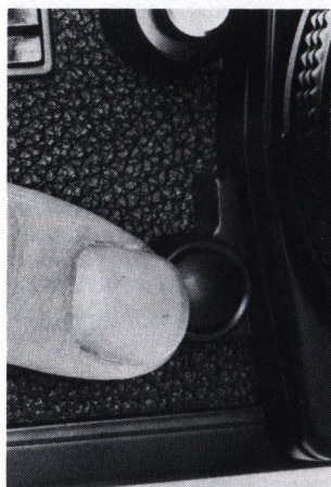
Exposure memory lock button allows close-up metering to be done on auto exposure and also holds exposure indication in finder. It's handy, but not when motor drive is attached.
