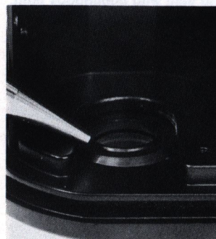
While it's not advisable to remove the motor drive from the camera when the camera is loaded, a spring-loaded light trap inside of film cartridge chamber does minimize danger of fogging (see text for fogging tests).
