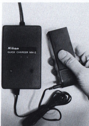
Alternative Nicad battery pack can be recharged in 3 hrs. and power entire camera even in cold temperatures.
