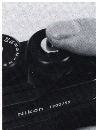
Electromagnetic shutter-release button is gentle and smooth, is threaded for traditional tapered cable release. Pressure on shutter release turns on metering circuit for approximately 16 sec., after which it goes off automatically if pressure is not maintained or renewed.
