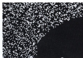
You can't see oval holes in F3's main mirror by just looking, but this backlit photomicrograph reveals part of the random, keyhole-shaped pattern.
