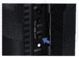
The self-timer has two release delays, 2 or 10 seconds. Choose  $\mathfrak{O}_2$  to minimize the risk of camera-shake in critical situations, or  $\mathfrak{O}^{10}$  to put yourself in the picture.
