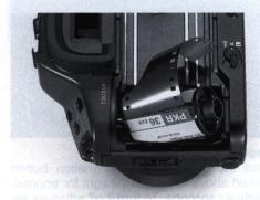
2) Insert the flat end of the cartridge into the top of the film chamber. The film cartridge symbol " appears in the display panel.
