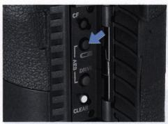
Open the palm door and press the battery check button.
