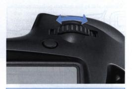
• When using non-DX film cartridges, the previously set film speed blinks in the display panel to warn that the correct film speed may not have been set. This warning stops after the two buttons marked "AF" and "METERING" on top of the camera have been pressed. If you want to change the ISO setting, turn the main dial while pressing these buttons.
