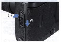
Open the back cover by pressing the back cover lock button in and sliding the latch down.
