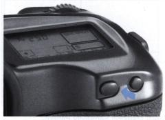
Lock the exposure by pressing the AE lock button on the back of the camera. The AE lock indicator \*\* appears in the viewfinder. Recompose the picture while keeping the shutter button pressed halfway.
