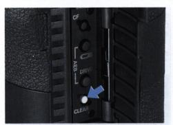
1) Open the palm door and press the white mode clear button, marked "CLEAR".
