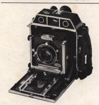
MANUFACTURER'S SPECIFICATIONS: Horseman Technical camera for 2½ x 3½ sheet film, 220 and 120 roll film. FEATURES: Interchangeable lens boards, interchangeable lens cams, rising, swinging and tilting front, swinging and tilting back, drop bed, built-in coupled rangefinder, multiframe viewfinder, swing-away infinity stops for each lens, adjustable leather strap handle, accessory shoe, dual tripod sockets. PRICE: With 105mm f/3.5 Professional Horseman lens and cam, \$399.50.
