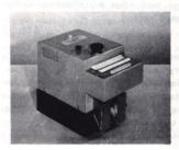
*†Kodak Slide Mounting Press,* Model 2-A compact and versatile press for large-volume mounting of color transparencies. Accessory removable jaws, supplied separately (see below), are available for use with the various sizes of transparencies. A numbering attachment to emboss numbers into the mounts is also available. 115-volt, 50-60-cycle ac.
