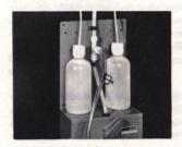
\*Kodak Chemical Replenishing Unit-For intermittent semiautomatic replenishment of measured quantities of a solution for use with Kodak Rack and Tank Color Film Processors, or with sink processing tanks. Ideal for film and paper reel processing, basket processing, or any system using intermittent or batch replenishment. Bottles must be ordered separately.
