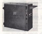
**†Kodak Versamat Film Processor**, Model 11A-M-For rapid, automatic, and controlled processing and drying of 4x5 through 11x14 black-and-white sheet films. With available accessories, listed below, accommodates continuous lengths of 16mm through 91/2inch-wide roll film. Stainless-steel construction. Automatic chemical replenishment and temperature control of solutions (at least 4 gallons per min-
