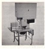
**†Kodak Roll Paper Printer, Type** IVB-3 (5x7) - Extremely versatile high-speed roll paper printer for making any size prints up to 7 inches long on roll paper up to 5 inches wide from any negative size up to 31/2 x5 inches. Ideal for "school," "wallet," and identification pictures, in black-and-white or color, using single or multiple lenses. Also readily adaptable to black-and-white 5x7-inch enlargements and 41/4- or 31/2-inch greeting cards from photofinishing negatives.
