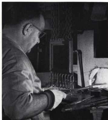
The glass cubes are heated to the softening point and molded into lens "blanks" in a special furnace.
