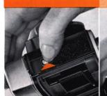
Open the back by pushing the LATCH BUTTON upward.
