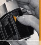
Open the back by pushing the LATCH BUTTON upward.
