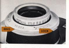
are using, then set this number on the camera as follows: Depress the selector ring LOCK and revolve the selector RING counterclockwise until the blue flash arrow snaplocks opposite the proper flash guide number on the lens mount (if impossible to set, change focus setting). A guide number of 70 is set in the illustration.
