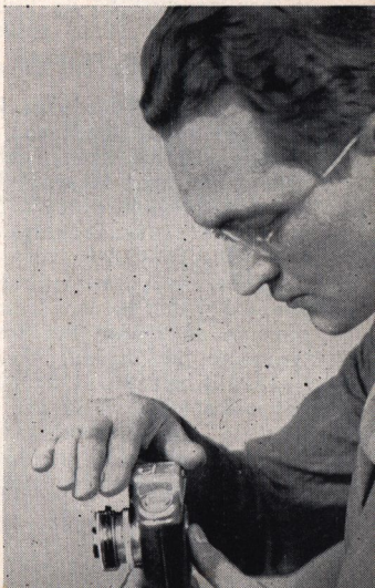
Fig. 7—Removing Exposure Meter from Colorcamera
