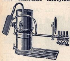
This Generator has the great advantage of portability, packing into a small box for carrying. It gives a very fine light equal to 150 candlepower, and when once started requires little or no attention. Owing to its construction it is easily cleaned. Lump carbide is used, and one pound will supply light for four burners for two hours.
