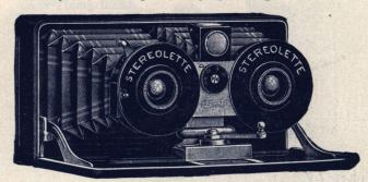
An exquisitely finished camera taking Stereoscopic pictures. It is made of metal, leather-covered, has a rising front and is rack and pinion focussing. The shutter is an everset automatic. A hooded focussing screen and two slides are supplied.
