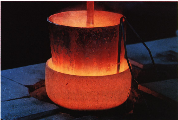
Ultra-purity is a prerequisite for melting superior optical glass. This melting crucible might well be one of the most valuable of its type. It is made of pure platinum.
