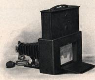
The front bed is fitted with a rack and pinion for fine focusing and the standard has a rising, falling and sliding adjustment.
