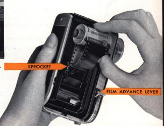
Drop the end of the film into the slot in the take-up drum. Hold down the edge of the magazine and move the film advance lever until the film is once around the drum. Close the back. Make sure it snaps in place. Move the film advance lever until the mechanism locks—this may require several full strokes of the lever.
