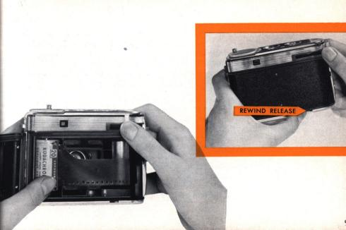
3 For the third time advance the film, as described above, until the mechanism locks—about 3 full strokes of the film advance lever.
