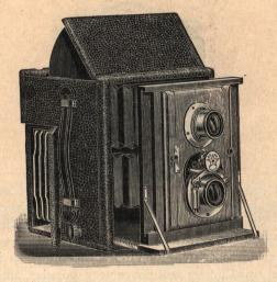
The CARLTON TWIN LENS CAMERA, as will be seen by the illustrations, is a divided camera, having two lenses of precisely the same focus, one placed above the other; the lower one forms the picture on the plate, while the upper one reflects the image on a ground-glass at the top of the camera.
