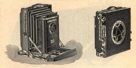
No Loose Top for Tripod.—The bed of the Carlton carries its own Tripod top, adapted to the Rochester Optical Co.'s Combination Tripod. The Top, made of metal, is neatly fitted in the bed and revolves easily and with great smoothness, permitting the operator to adjust the Camera in any direction. A small milled head secures it firmly in position.
