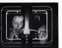
instance, the standard lens (dotted in the illustration) as the upper limit of the field of view at 2¾ feet. At distances beyond 2¾ feet this limit gradually moves upwards, until it coincides with the edge of the line frame itself for subjects at 8 feet and over.
