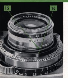
The front component of the RETINA lens is interchangeable. To remove the standard lens, rotate it anti-clockwise as far as it will go, and lift out of the shutter. We recommend the use of the special lens container designed for the standard lens for easy changing and convenient storage.
