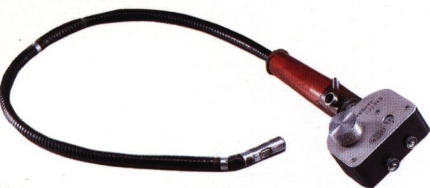
The world's first gastrocamera (for taking photographs inside the stomach)
