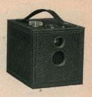
For square pictures  $3\frac{1}{2}$  x  $3\frac{1}{2}$  inches; capacity, 12 exposures without reloading; size of camera,  $4\frac{1}{2}$  x  $4\frac{1}{2}$  x  $5\frac{1}{2}$  inches; weight, 19 ozs.; length of focus of lens,  $4\frac{1}{2}$  inches.
