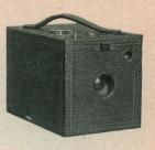
For square pictures  $3\frac{1}{2}$  x  $3\frac{1}{2}$  inches; capacity, 12 exposures without reloading; size of camera,  $4\frac{1}{2}$  x  $4\frac{1}{2}$  x  $6\frac{1}{2}$  inches; weight, 28 ounces; length of focus of lens,  $5\frac{1}{2}$  inches.
