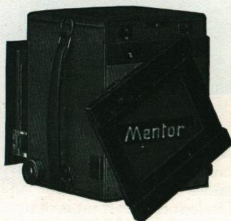
The small Mentor is a box form square Reflex camera with a reversing back for upright and landscape pictures. It is made only for  $3\frac{1}{2} \times 2\frac{1}{2}$  ins. ( $6\frac{1}{2} \times 9$  cm.), and so the body of this camera measures but  $5\frac{1}{8} \times 4\frac{3}{4} \times 6\frac{1}{4}$  ins. Fitted with Zeiss lenses f 4.5.
