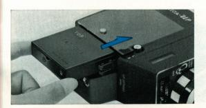
Place the holder back in the base of the camera with the terminals and 'TOP' mark pointing upwards, and replace the cover.
