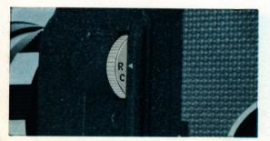
Turn the Aperture Dial towards the smallest lens opening until "R" is in a position opposite the triangle, thus, the film will be released for rewinding.
