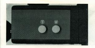
Two zooming buttons are located on top of the camera. Full operating time for zooming from Wide Angle to Telephoto and Telephoto to Wide Angle is approximately 3.5 seconds. Before operating, note focal length set on lens mount and then press appropriate button. While filming a zoom sequence, both shutter release button and zooming button must be pressed simultaneously.
