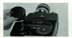
Flim must run along the white arrow-line film-path marked inside, with the white (emulsion) surface of the film facing out (toward the lens).
