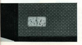
Note the position of the footage counter, then turn the lever slowly and rewind the film to the desired length by closely watching the footage. Do not rewind the film when the remote control is used.
