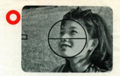
While looking through the viewfinder turn the distance scale ring either clockwise or counterclockwise until the upper and lower portions of the image are seen in the circle into perfect alignment.
