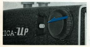
To check the meter, set the Frame Speed Dial at 16, then press in on the Power Button and read the needle in the indicator.
