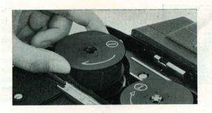
■ Open the side cover, remove the loaded spool (on which the exposed film has been wound) from the take-up spindle, taking care not to loosen the film.
