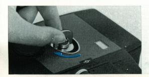
Close the side cover and turn the lock clockwise to lock it.
