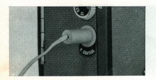
Insert plug of the controller cord into the remote control jack. (Located below the Frame Speed Dial.)
