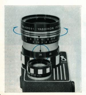
Critical focus through the viewfinder is necessary before filming your subject. Once the subject has been brought into clear focus by rotating the focusing ring, distance scale ring change is not necessary while zooming.
