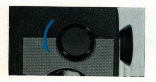
Unscrew the cap for the Rewind Lever.
