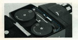
Holding both spools, place the loaded spool on the upper spindle, the empty one on the lower spindle, and insert the film along the arrow-path into the film gate.
