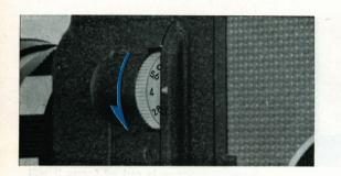
Before filming, be sure to check the condition of batteries if they are in good condition by reading the Power Indicator. The aperture dial must be off the "AUTO" position.
