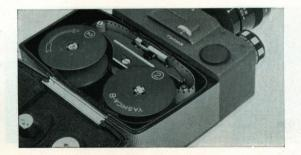
Turn over the loaded spool so that the ② is visible, and then insert it in the upper spindle.
