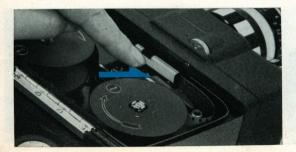
Close film gate with your finger and press the Shutter Release Button for two seconds as a test for smooth film movement. The film gate automatically closes when the cover is locked.
