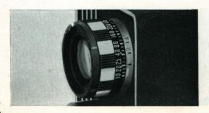
Proper exposure of these scenes may be obtained, automatically, by simply setting the ASA speed of the film in use opposite the number 2 on ASA control ring of the exposure meter. Remember to reset ASA speed index of the film opposite the triangle mark for normal scenes after use.
