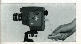
Note: Unless the Shutter Release Button is depressed and locked, the remote control system does not work, even if the switch is turned on.
