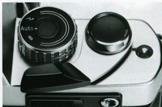
Unique feather-touch electromagnetic release button on hub of film wind lever. Film advance lever unlocks the exposure check button on full return. Shutter control dial has only "AUTO", "B" and " \lambda " (for flash) settings to offer utmost convenience in operation.
